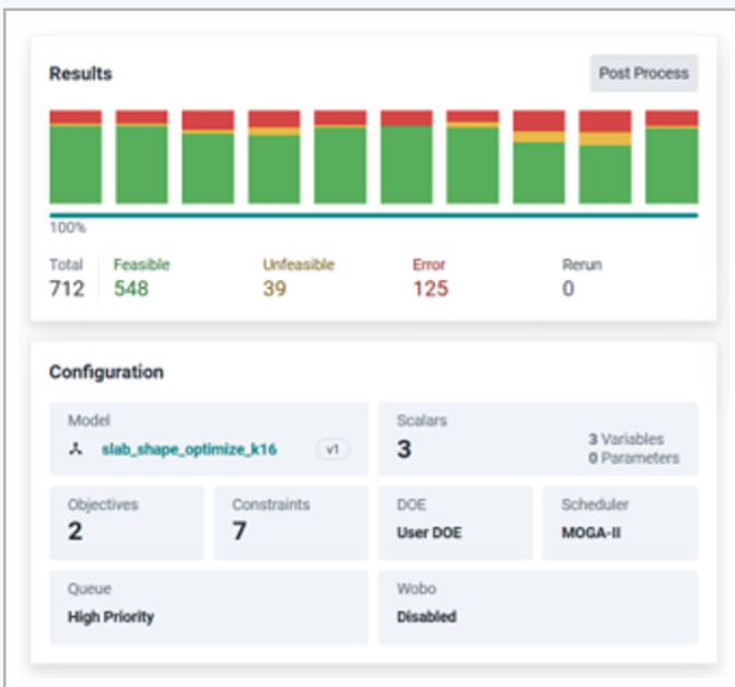
The session with the summary of VOLTA Planner configuration, a modular environment to apply several optimization strategies, shows the set-up and execution results of the design space exploration plan chosen to optimize the shape of the all structure.
