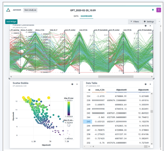
VOLTA Advisor, the advanced data analysis web environment, allowed to assess simulation results and choose the optimum design with minimized both the building weight and the maximum displacement of slab.
