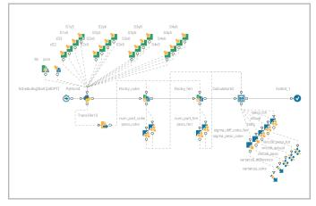
The workflow set up in modeFRONTIER to automate the simulation process in Rocky DEM and run the design optimization strategies.
