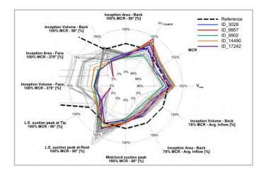
"Starting from a set of 48 blade parameters to alter the reference propeller geometry, the use of MOGA-II algorithm allowed to compute and test 50,000 different geometries in about 5 days to achieve a satisfactory **Pareto convergence** and choose optimal candidates (one for any rake distribution) for RANSE analyses" said **Michele Viviani, Associated Professor at DITEN Department, Genoa University**.
